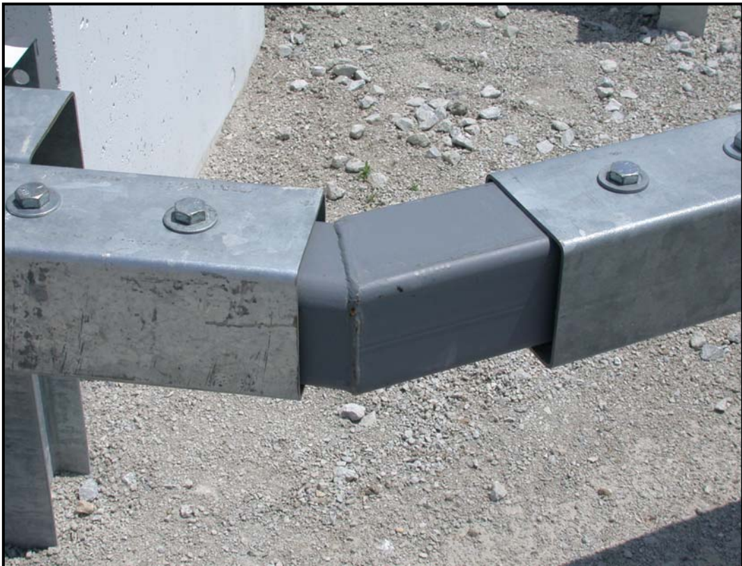
Figure 10. Bent Splice Connection for BEAT-BP
