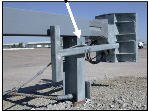
Figure 14. Impact Head, Post #1, Post Breaker, Tether Cable for BEAT-BP
